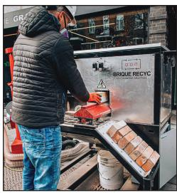
Three years in the making, the patented machine cleans 99 per cent of a brick through a process involving a concrete grinder that allows the cleaning of the brick extremities.
